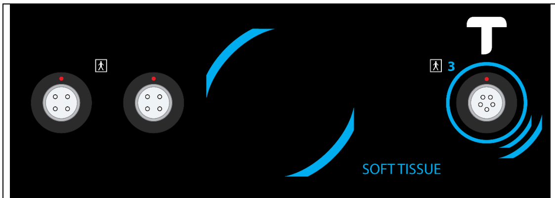
Figure 14 Soft tissue transducer – high power selected
